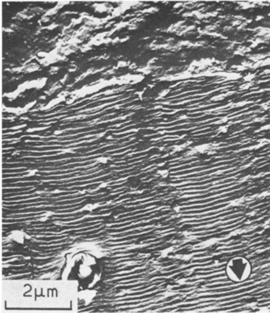
Figure 5 Fatigue-crack growth of an aluminium-copper alloy in vacuum, followed by growth in air. Carbon replica illustrating the effect on striation visibility [34]. (Courtesy American Society for Metals.)
